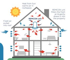
Slightly increased air pressure pushes out moisture via gaps in doors, windows & air bricks that would have formed condensation and black mould
